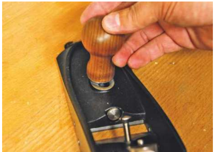
▲ Slackening the front handle adjusts the mouth for finer work
